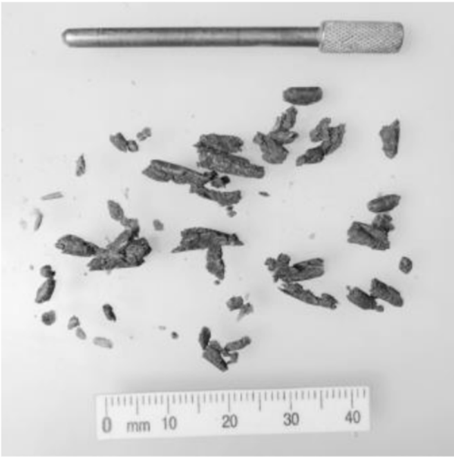
FIG. X2.1 Example of Soil at the Plastic Limit
