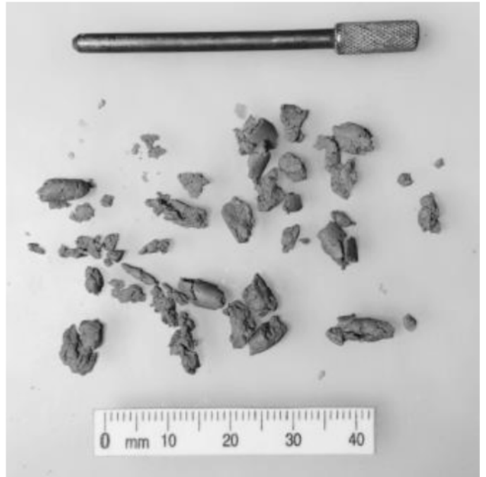
FIG. X2.3 Example of Soil at the Plastic Limit
