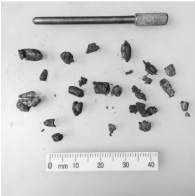
FIG. X2.2 Example of Soil at the Plastic Limit
